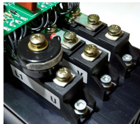
Showing the position of the bus-bar, linking on the supply inputs, (L1, L2 and L3) side of the thyristor Paks on units of 5.5kW through 37kW.
