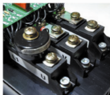
Showing the position of the bus-bar, linking on the supply inputs, (L1, L2 and L3) side of the thyristor Paks on units of 5.5kW through 37kW.
