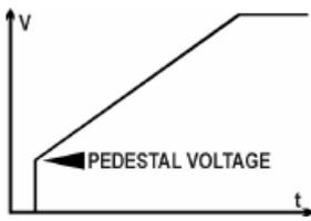
This sets the initial voltage that is applied to the motor. This is adjusted to a level so that the motor starts to accelerate smoothly and immediately.
