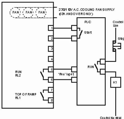
1. The **EnviroStart** will start as soon as K1 closes and then “start” is made. The **EnviroStart** will stop when “start” is opened.
