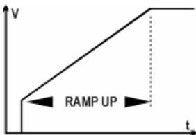
The Ramp Up switches adjusts the time from the initial Pedestal setting to full output voltage. Switch settings as follows:
