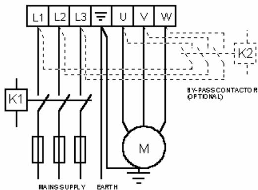
NOTE: IF POWER FACTOR CORRECTION CAPACITORS ARE FITTED THEY MUST BE PLACED ON THE LINE SIDE OF K1 AND MUST NOT BE SWITCHED IN OR OUT WHILE ENERGY CONTROL IS RUNNING.
