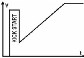
On some high stiction (high static friction) loads, a better mechanical start can sometimes be achieved by using the Kick Start feature to overcome the resistive torque.
