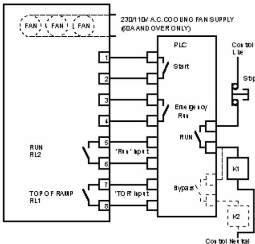
1. The unit will start as soon as K1 closes and then “start” is made, The **EnviroStart** will stop when “start” is opened.
