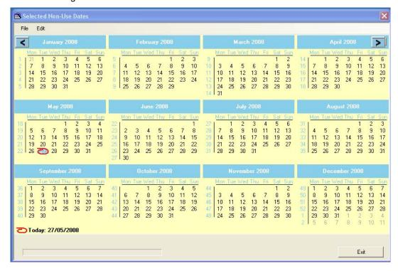
Selecting Non Use Dates allows you to utilise the onboard ten year calendar to tell the **LPTimer** to shut off the motor for a given day irrespective of what is selected in the Run Times described above. This would allow for the exclusion of use on public holidays for example or factory shutdowns.
