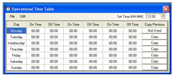
You can set the start and stop times for the **LPTimer** manually if required, by using the "Set Time" function to the top right of the window or if you highlight an "On Time" and then right click with the mouse you will call up the "Time Select Slider" window which allows you to input start and stop run times visually.
